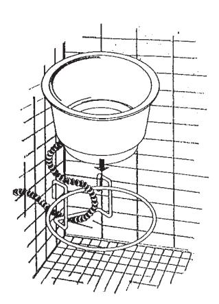
**Wooden Surface Installation** You may also mount hutch bracket on a wooden surface. Use two "U-shaped" nails or staples as shown in diagram below.
